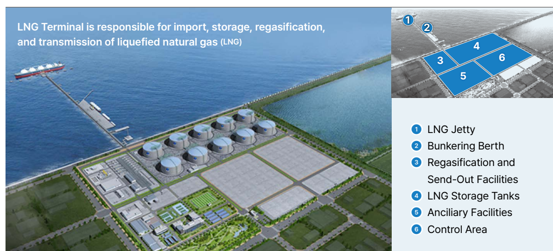
[Figure 3] Structure of LNG Terminal
